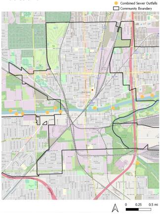
Above is a map of all the combined sewer outfalls the Metropolitan Water Reclamation District has identified near Blue Island. Combined sewer outfalls are utilized when sewer systems are at capacity and so rainwater is discharged (emptied) directly into a water body to reduce flooding. These discharges can have bacteria or other microbes that can lead to illness, so it is important to be careful around these water bodies.
